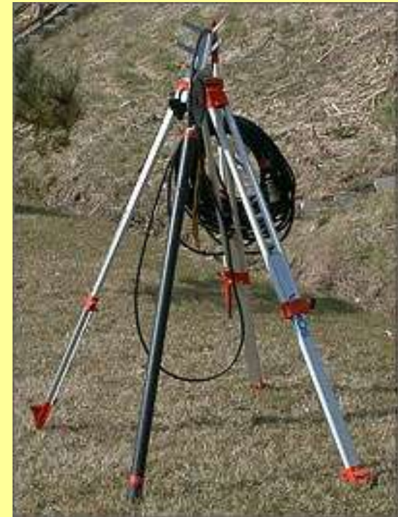
Bore Hole Antenna with Tripod and Survey Wheel
