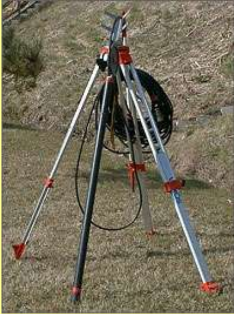
Bore Hole Antenna with Tripod and Survey Wheel
