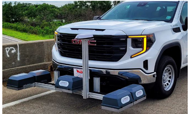
LTRC researchers recommend the SAG inertial profiler (pictured above) be employed for pavement evaluation across Louisiana.
