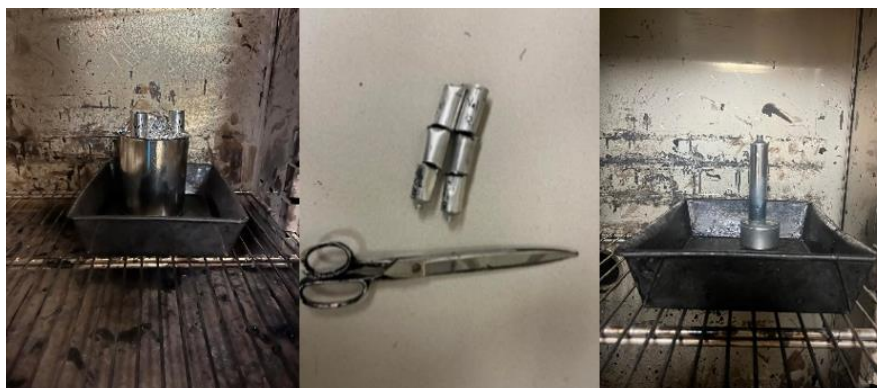
Figure 2. Storage stability: cigar tube at conditioning, aluminum tube cutting, and retrieving EA binder from aluminum tubes
