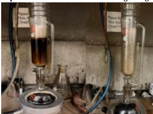
Figure 3. Soxhlet asphalt extraction: thimble at the beginning and end of the test
