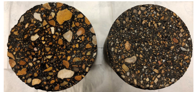
Figure 1. 12.5-mm (left) and 4.75-mm (right) NMAS mixtures
