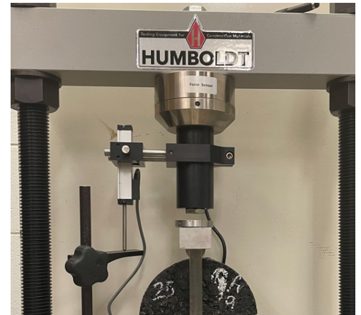
Figure 1. SCB Test Setup
