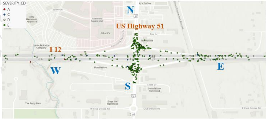
Figure 80. Distribution of all severity levels at Interchange 6
