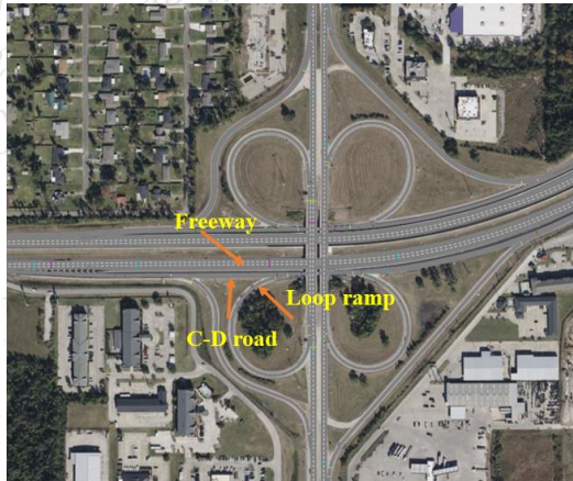
Figure 30. Cloverleaf interchange without C-D roads
