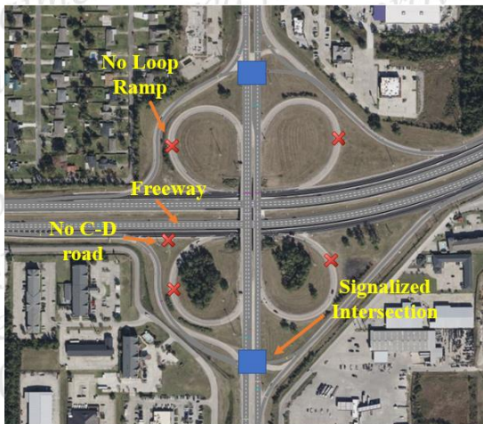
Figure 31. Diamond interchange with signalized intersections
