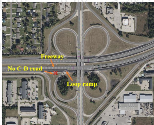
Figure 30. Cloverleaf interchange without C-D roads
