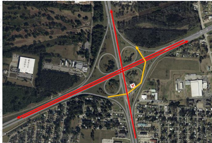
Figure 14. Recommended modification after 20 years at Interchange 2
