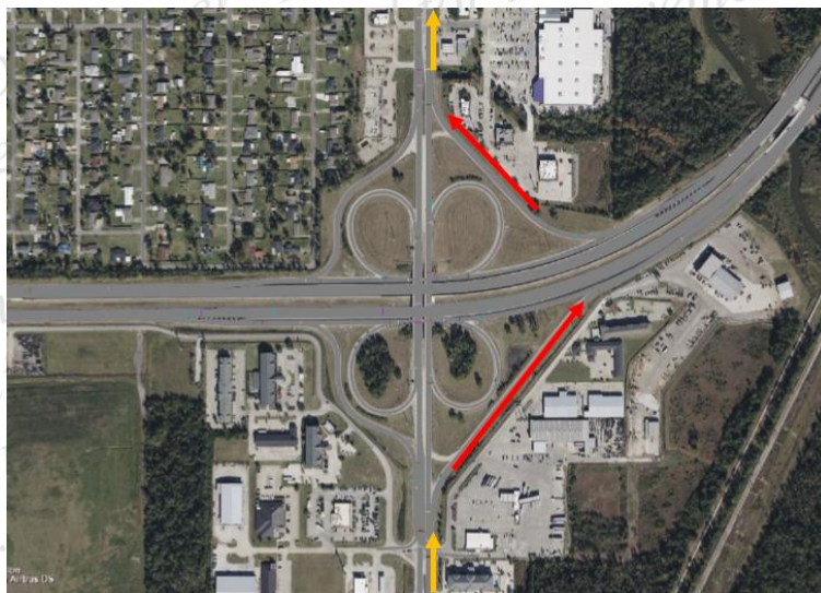
Figure 11. Recommended modifications after 20 years for Interchange 1
