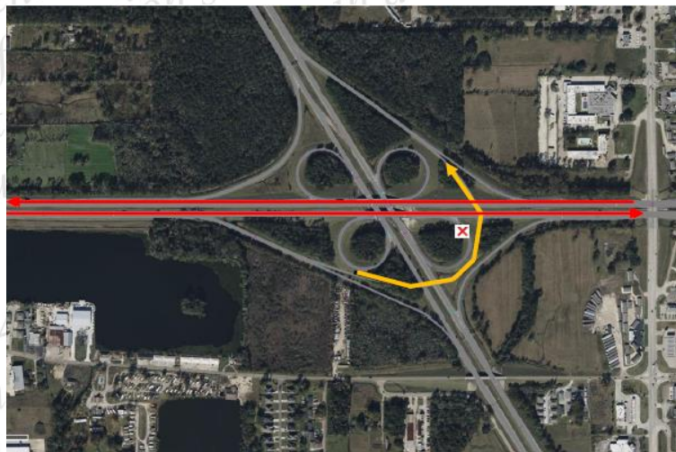
Figure 18. Recommended modification after 20 years for Interchange 3
