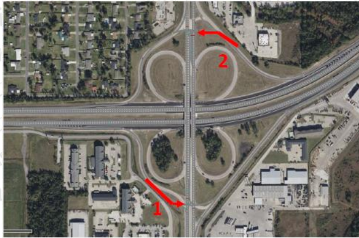
Figure 34. Left turn traffic movements at Interchange 1
