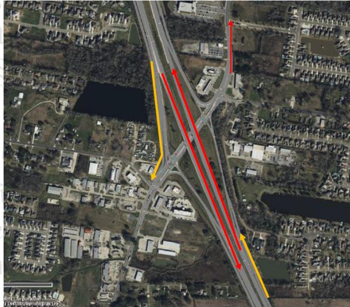
Figure 26. Recommended modifications after 10 years for Interchange 7
