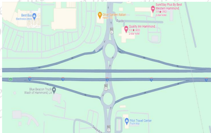
Figure 57. Interchange 6 (Diamond with double roundabouts)
