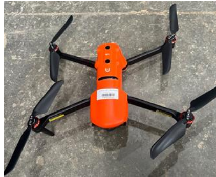
Figure 6. Autel Evo II pro V3 UAV used for data/image collection
